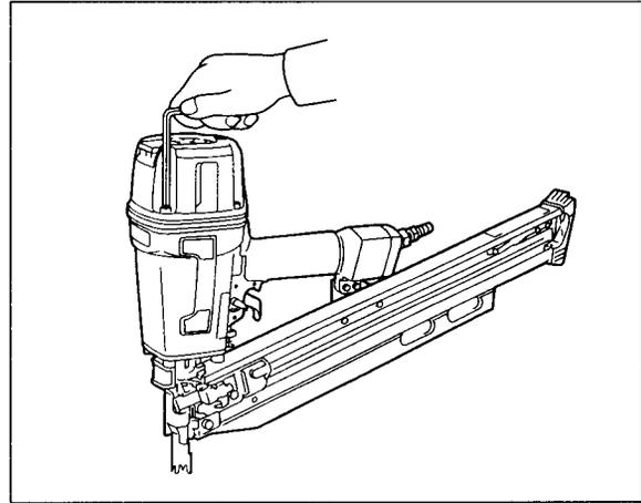
With tool disconnected, make daily inspection to assure free movement of the contact element and trigger. Do not use tool if the contact element or trigger sticks or binds.
